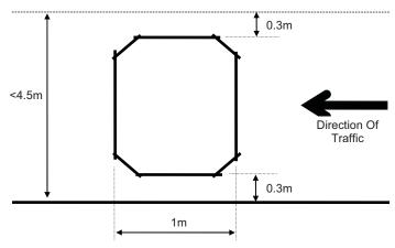
The sensing loop consists of n turns of cable indicated as follows:
