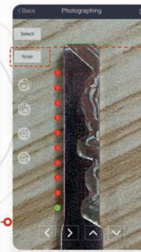
Step 7 Adjust the key picture in designated area by clicking "Rotating" / "Zooming" / "Moving" button
