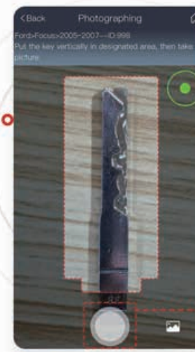
Step 6 Put the key vertically in designated area, then take a picture
