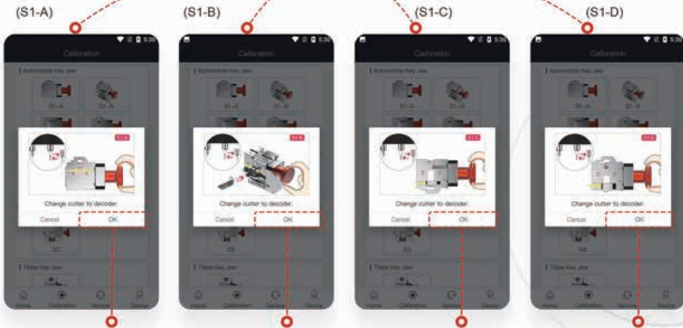
Step 3 Change cutter to decoder, place the calibration block and fix jaw tightly, then click "OK" button shown as picture
